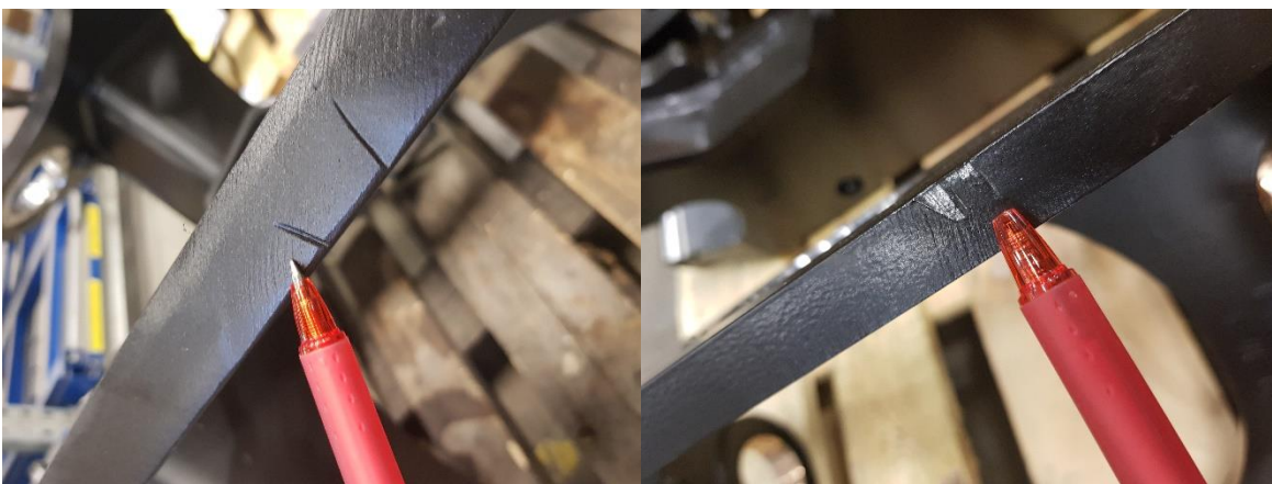
Example not permitted damages
